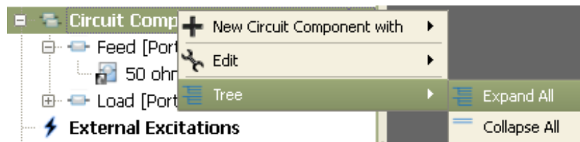
Figure 4.24: Expanding and collapsing all branches in the Project Tree
