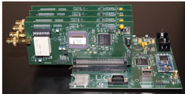
Figure 27: The ARIANNA data acquisition system triggers and digitizes simultaneously the analogue waveforms [6].
