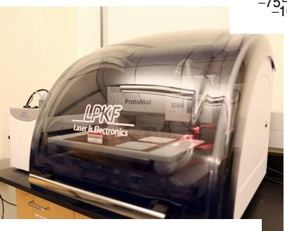
Mill machine for Radio circuit boards
