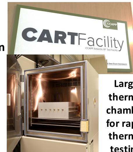
Large thermal chamber for rapid thermal testing
