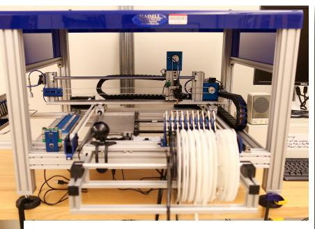
Pick & Place Machine for rapid mass assembly
