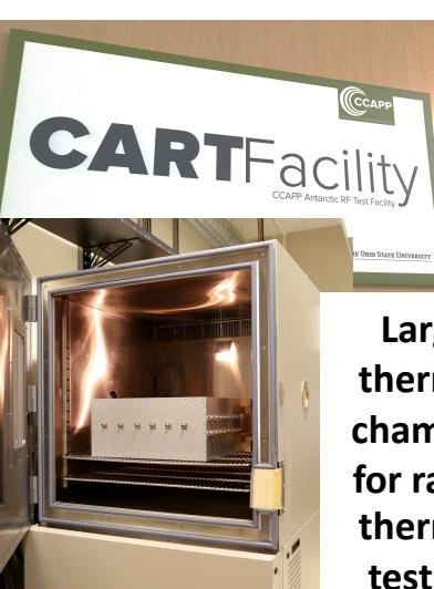
Large thermal chamber for rapid thermal testing
