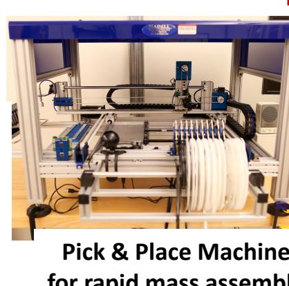
Pick & Place Machine for rapid mass assembly
