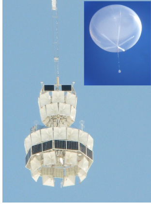
FIG. 9: A look at the final product of ANITA-II. The inset is a picture captured during the flight, with the balloon between 33-35 km above the surface of the Antarctic. Image from [22].
