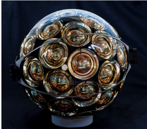
Figure 4: A picture of the KM3NeT DOM. Each bronze circle is an exposed photocathode from one of the 31 PMTs. The small circle just left of the center is the DAR. Image and description adapted from [37].
